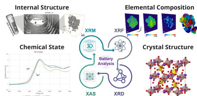
Figure 1: Non-destructive x-ray techniques in battery research.
