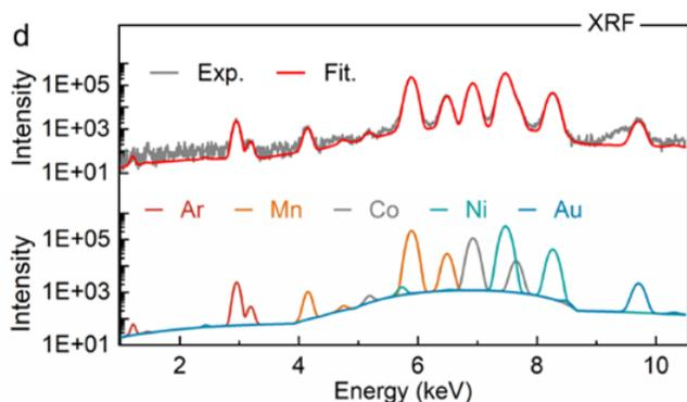
**Figure 7:** Identification and quantification of elemental composition in a micron-scale spot of an NMC battery using AttoMap's intuitive software. Relative weight percent or absolute amounts can be calculated using models or standards.
