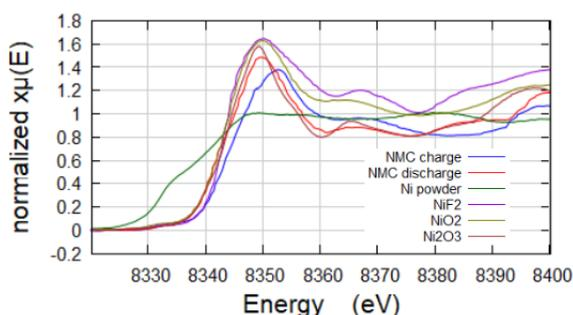
**Figure 3:** Example of QuantumLeap spectra, in which absorption of x-rays are plotted as function of their energy. Shown are 6 spectra of Ni: charged and discharged NMC batteries and reference foils (Ni, NiF<sub>2</sub>, NiO<sub>2</sub>, Ni<sub>2</sub>O<sub>3</sub>).
