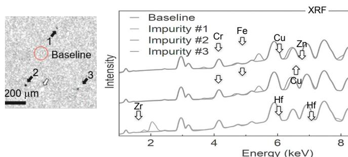
**Figure 8:** Correlative study using x-ray imaging followed by microXRF on the AttoMap to quantify the distribution of Ni, Mn, and Co in an NMC battery and to identify particulate impurities (Fe, Cr, Cu, Zn, Zr, and Hf) produced during battery production [8].
