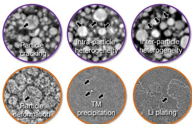
**Figure 17:** *In situ* characterization of multiple structural degradation mechanisms of batteries during cycling, including: particle deformation, particle cracking, transition metal precipitation, Li plating, and dendrite formation and growth using Apex XCT.
