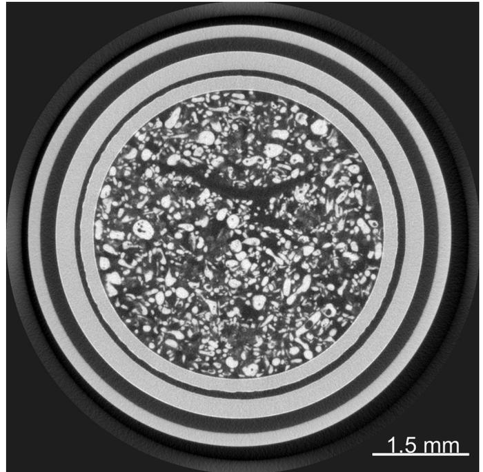
Figure 14: Commercial LICB LR626 coin cell (horizontal cross-section)
